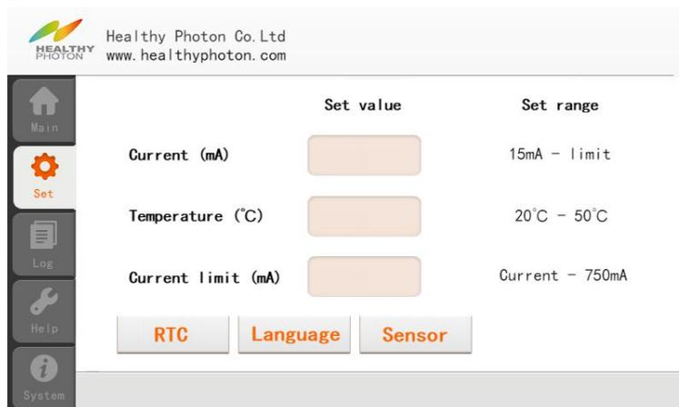
Check whether the set value of NTC thermistor is the same as the thermistor used in the laser package. If they are different, click the Sensor button to choose the right thermistor. For example, press [OK] to switch the thermistor from 20 K $\Omega$  to 10 K $\Omega$  as shown in the following screenshot:
